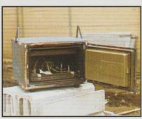
Test Result: After these tests, upon opening, the contents of the safe remain intact as expected-even the colour of the papers did not change.
