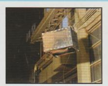
Dropping Test: The safe is then subjected to a drop and impact test. It is dropped from a height of 4 meters to simulate a situation where the safe might fall
